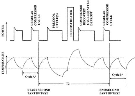
$^{\circ}$  Average compartment temperature during cycles A & B must be within 0.5 F of the average temperature for the first part of the test.
