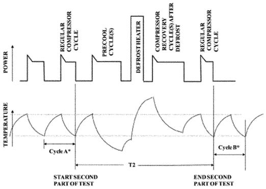
\*Average compartment temperature during cycles A & B must be within 0.5 F of the average temperature for the first part of the test.
