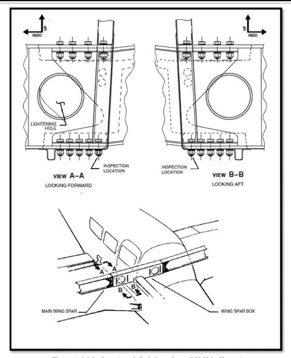
Figure 1. Main Spar Attach Bolt Locations (RH Side Shown)
