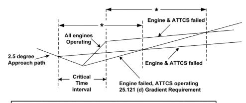
\* The engine and ATTCS failed time interval must be no shorter than the time interval from the point of simultaneous engine and ATTCS failure to a height of 400 feet used to comply with I25.2(b) for ATTCS use during takeoff.
