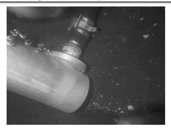
Photo 2 – Leak at left ATF port from submerged cooling cylinder
