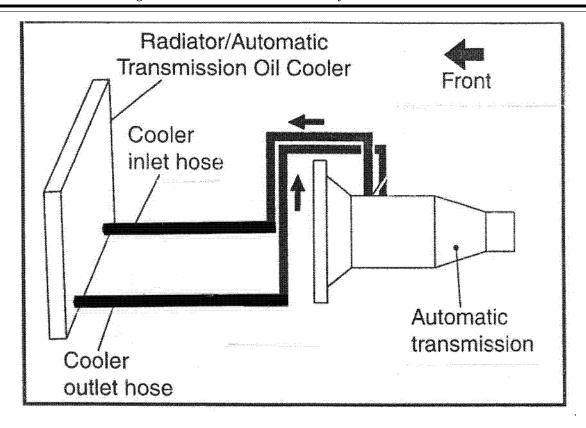
Figure 1 – Subject transmission cooling system - fluid flow schematic
