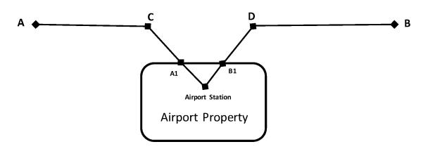
• The approximate incremental cost to serve the airport is the difference between the track cost to serve the airport (C-A1-Station-B1-D) and the cost if the track did not deviate to serve the airport (C-D). This incremental cost represents the costs needed to directly benefit airport passengers and employees. This incremental cost forms
