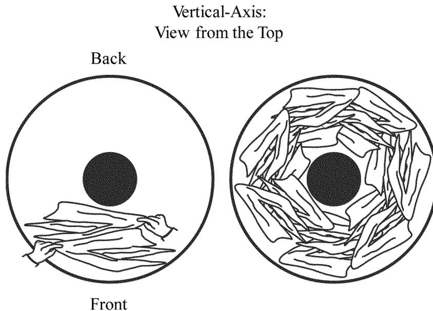
**Figure 2.9.2.3—Loading Energy Test Cloths into a Front-Loading Clothes Washer**
