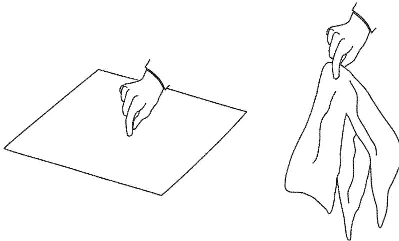
To load the energy test cloths in a top-loading clothes washer, arrange the cloths circumferentially around the axis of rotation of the clothes container, using alternating lengthwise orientations for adjacent pieces of cloth. Complete each cloth layer across its horizontal plane within the clothes container before adding a new layer. Figure 2.9.2.2 of
