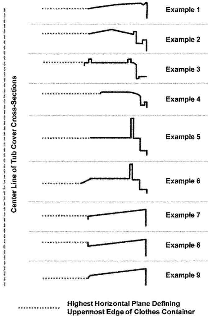
For a front-loading horizontal-axis clothes washer, fill the clothes container to the highest point of contact between the door and the door gasket. If any portion of the door or gasket would occupy the measured volume space when the door is closed, exclude the volume that the door or gasket
