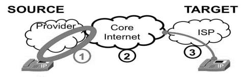
= 100 ms round-trip measurement Or 50 ms one-way – edge-to-core (designated IXP) = Carrier + Transit Tier II & III to IXP
