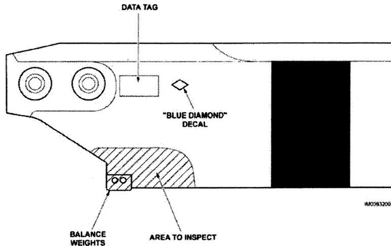
**Figure 1. Tail rotor blade inspection.**
