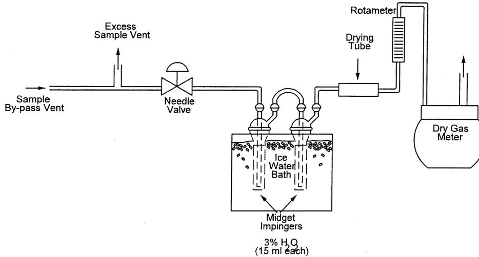
**Figure 6C-1. Interference Check Sampling Train.**
