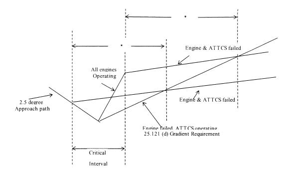
\* The engine and ATTCS failed time interval must be no shorter than the time interval from the point of simultaneous engine and ATTCS failure to a height of 400 feet used to comply with 125.2(b) for ATTCS use during takeoff.
