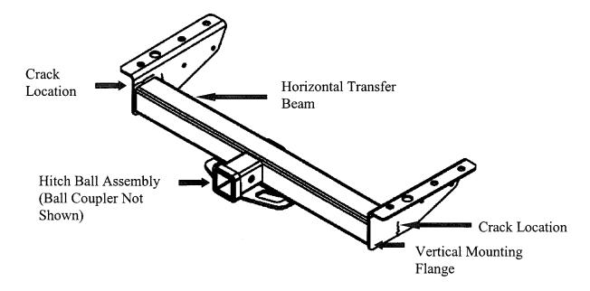
Figure 1. Typical Class III/IV towing Hitch Receiver
