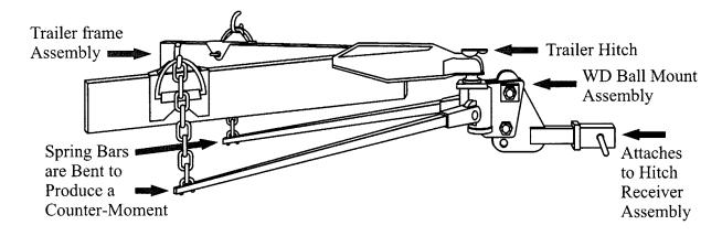
Figure 2. Typical Weight Distributing Hitch System Setup
