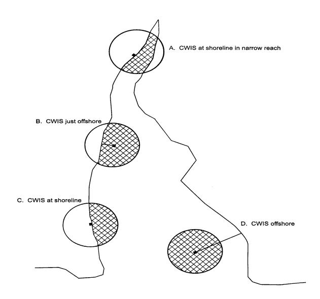
CWIS = Cooling Water Intake Structure
