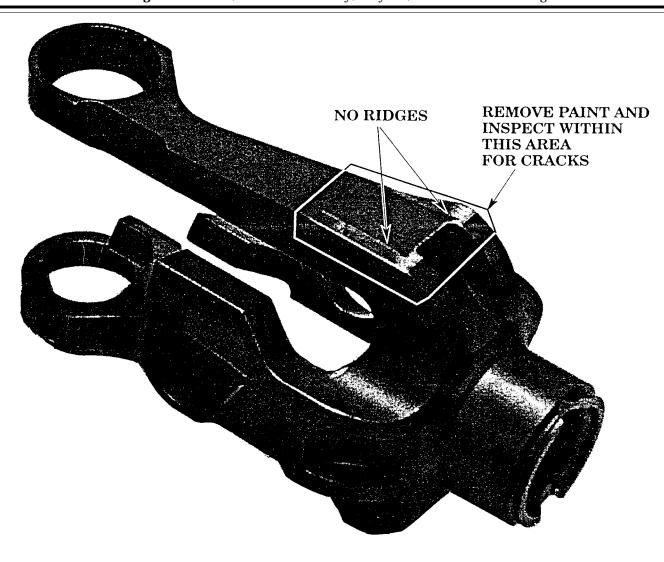
Figure 1. Fork Assembly without ridges (Sheet 2 of 2).
