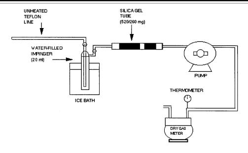
Figure 308.1. Sampling train schematic
