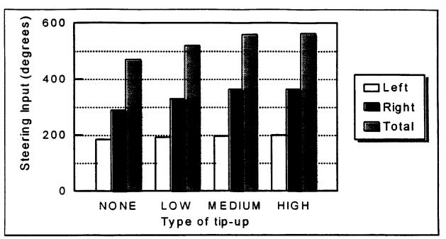
Figure 4. Average Steer Input for CU Tests of Subject Vehicles by Tip-up Result (November 25, 1996 submission).
