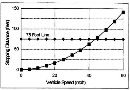
Figure 5. Stopping Distance vs. Vehicle Speed.
