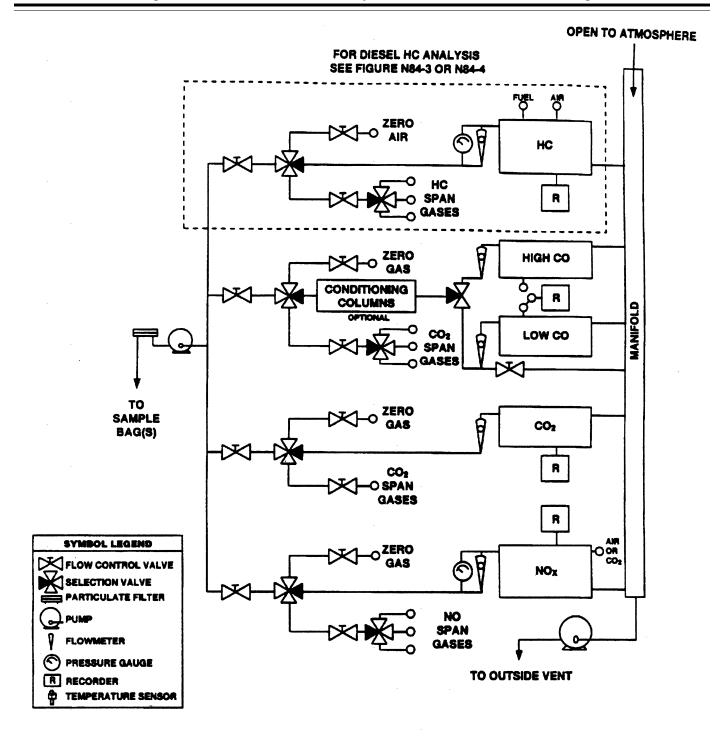
Figure 4. — Exhaust Gas Analytical System
